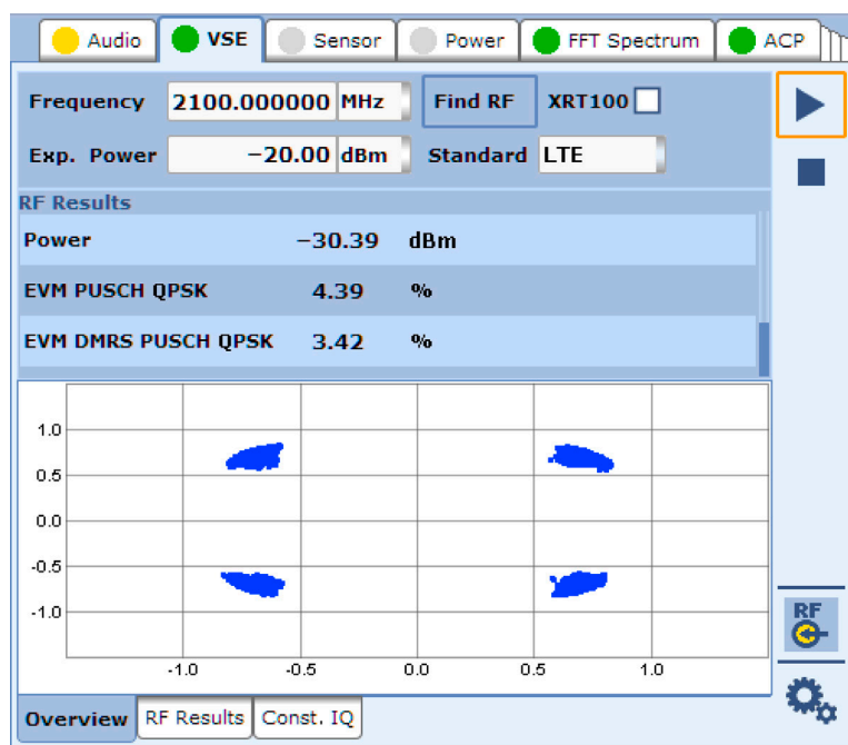
LTE transmitter measurement.
